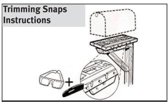
After you have Secured mailbox to Mounting Bracket you may, if necessary, trim the snaps off of the Mounting Bracket. To do this be sure to wear Safety Googles. Then carefully cut snaps off with a razor blade as shown in Illustration.
