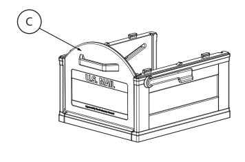
With the door open, place the roof onto the (2) side panels of the mailbox.
