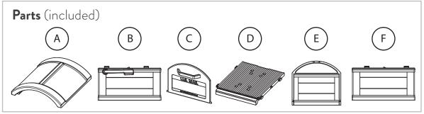
Place the right side and left side panels onto the floor panel where the locking tabs of the floor fit into the pockets of the side panels. Slide the panels to snap-lock into place.
