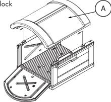
4 Slide the back panel into the back of the mailbox until fully snapped into place.
