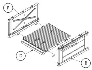
2 Insert the door by placing the hinge peg into the hinge hole of a side panel and rotating the second peg into the opposite side panel.
