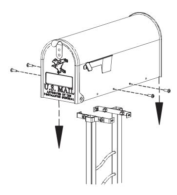
Check for underground cables or pipes before digging. Dig a hole measuring 12" deep and 8" in diameter. Place the mailbox post assembly in the hole. Replace and pack down the dirt around the post making sure the assembly remains level.
