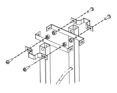
Attach mailbox (not included) to the post assembly using (4) screws and (4) hex nuts.
